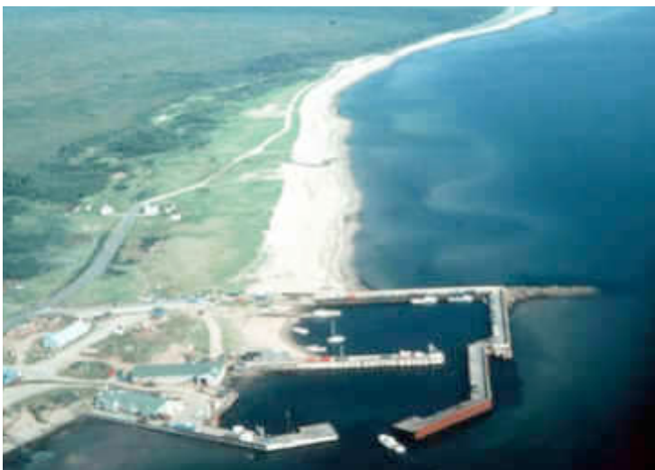
Figure 5. Trapping of sand behind a harbour in Richibucto Cape, NB.
